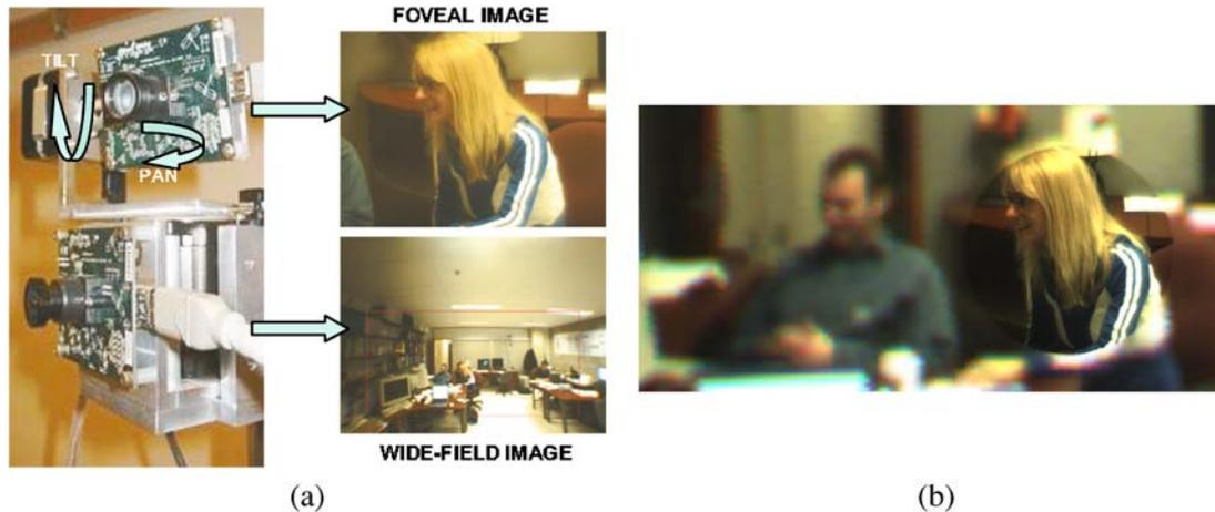
Figure 1. (a) Attentive wide-field sensor. (b) Fused output from the two sensors.
