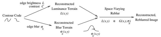
Figure 6: Inverting the contour code. Perceptually accurate reconstruction requires contour brightness, contrast and blur coding. Luminance and blur terrains are reconstructed and then combined by space-varying convolution.
