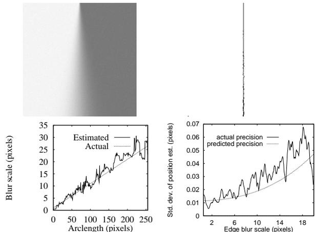
Figure 3: **Top left:** The blur grade is linear, ranging from  $\sigma_b = 1$  pixel to  $\sigma_b = 26.6$  pixels. Parameters (see Eqn. 1):  $A = B = 85$  grey levels,  $\sigma_b \in [1, 26.6]$  pixels,  $\sigma_n = 1.6$  grey levels. **Top right:** Edges detected by local scale control. **Bottom left:** Estimated blur scale  $\sigma_b$ . **Bottom right:** Predicted and measured localization precision  $\Delta x$ .
