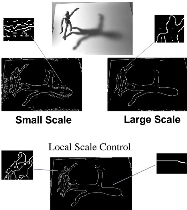
Figure 1: **Top:** Output of Canny edge detector for different filter scales. **Bottom:** Edges recovered by local scale control.
